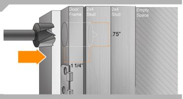
Use a 3/4" wood bit to drill into the door jam to a 1 1/4" depth.
