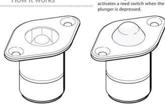
NOTE: The sensor typically protrudes .060" beyond the door jamb. Protrusion may vary slightly.
